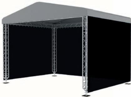
The MILOS MRO NGW 6x5m aluminium roof incorporates our HD Multi-Cube, eliminating the need for any wires or corner braces for this set-up. Using HD Multicube in the construction of this roof allows loading capacity of up to 30 kg/m plus 200kg for the PA. Great size, simple set-up, no hassle.
