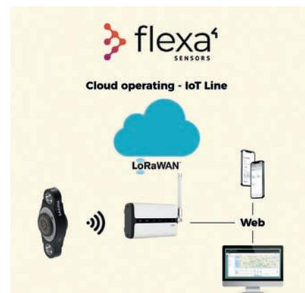
Each cell transmits its data to the nearest gateway which sends it directly to the cloud via the Internet. Those who have the credentials to log into the Flexa portal can access the information defined by their login status. The portal can be reached from a browser or from an app, for mobile devices. The portal allows different levels of permissions. For example, the installer can check his own
